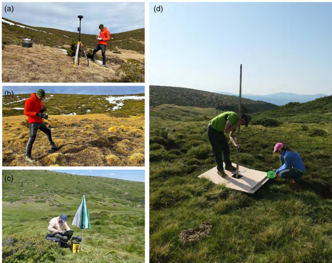
**FIGURE 3** (a) UAV flight using a D-RTK GNSS station and a DJI Phantom 4-RTK system. (b) Thermal surveying using a FLIR camera. (c) Geoelectric tomography surveying and (d) drill-core tasks. [Colour figure can be viewed at [wileyonlinelibrary.com](https://onlinelibrary.wiley.com/doi/10.1002/ldr.4968)]
